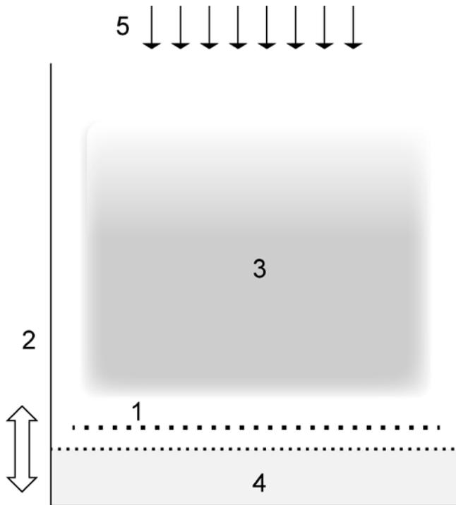
**Fig. 1.** Scheme of the reactor: 1 – the RF electrode, 2 – the reactor wall, 3 – the plasma-dusty cloud, 4 – the system for dispersion and collection of the powder, 5 – flow of Co atoms from a magnetron sputter. The arrows in the lower area of the figure point out to the direction of the reactor vibration in a powder dispersion process.
