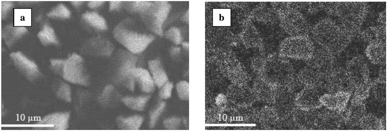
**Fig. 2.** Microstructure of the diamond powders with a cobalt coating. X-ray point images corresponding to carbon (a) and cobalt (b) demonstrate relatively homogeneous distribution of cobalt on diamond particles.
