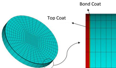
Figure 2. Finite element model of the experimental sample
