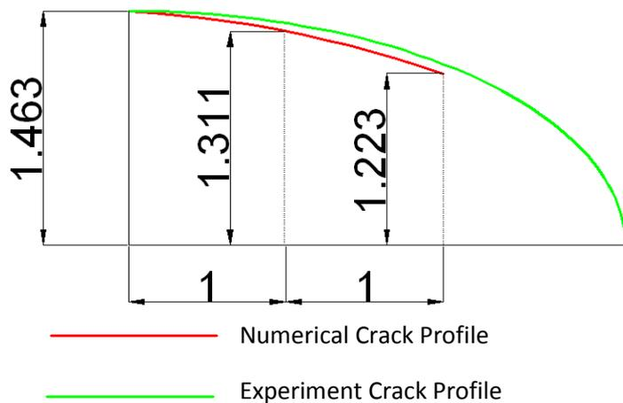
Figure 4. Crack profiles obtained experimentally and calculated numerically
