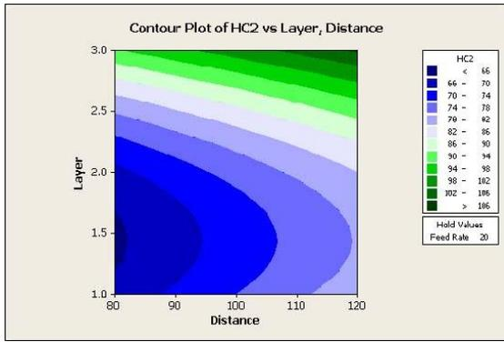
Figure 1: Cantour plot of hot corrosion resistance vs. standoff distance and number of layers.
