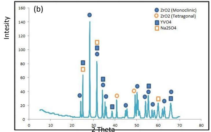
Figure 3: XRD patterns (a) before and (b) after hot corrosion tests at 800°C.
