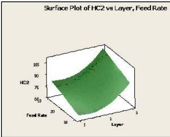
Figure 2: Surface plot of hot corrosion resistance vs. Feed rate and number of layers.
