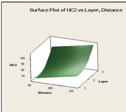
Figure 5: Surface plot of hot corrosion resistance vs. number of layers and standoff distance.
