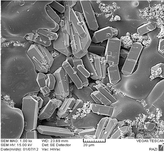
Figure 4: SEM picture for surface of coating after corrosion test.
