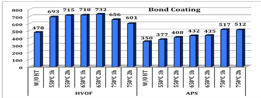
Figure 5. Microhardness results of the bond coatings for heat treated and without heat treated coatings
