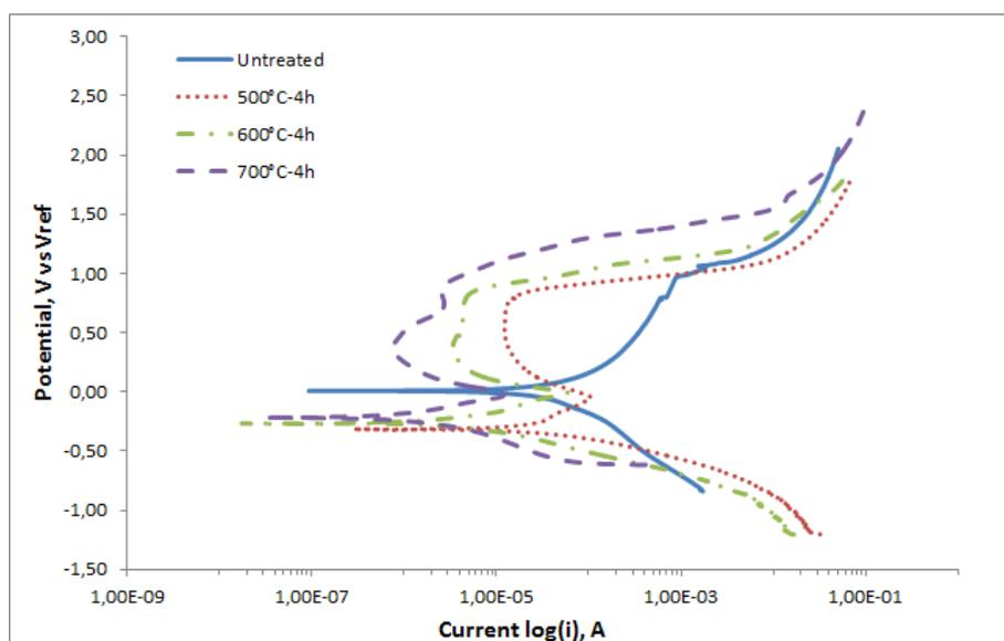
**Figure 3.** The potentiodynamic scan curves of specimens oxidized for 4h
