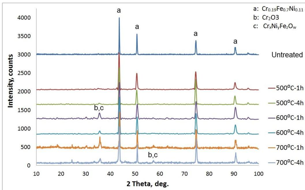
**Figure 1.** The XRD patterns of untreated and oxidized Inconel 718
