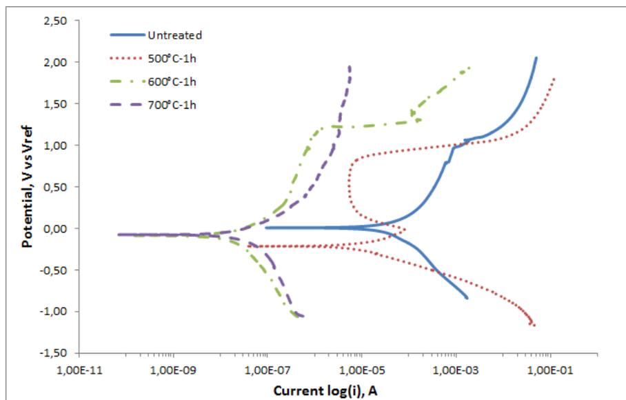
**Figure 2.** The potentiodynamic scan curves of specimens oxidized for 1h
