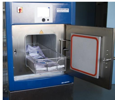
Figure 4: commercial sterilizer with integrated PLExc ® plasma source
