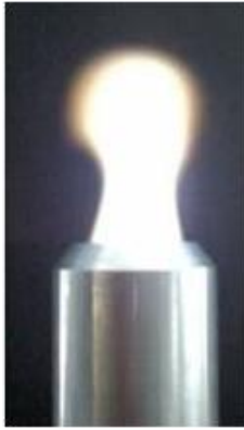
Figure 1: microwave excited plasmasource PLExc ® developed by INP
