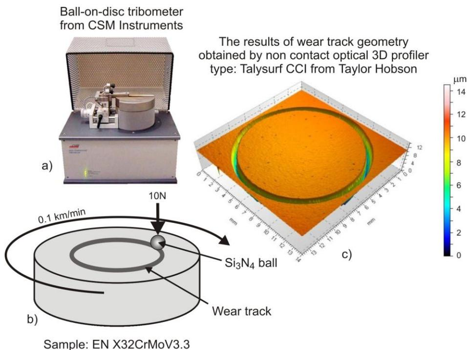
Fig.3. Realisation of ball-on-disk tribology tests: a) ball-on-disk tribometer from CSM Instruments, b) ball-on-disk tribology system, c) wear track geometry obtained by non contact optical 3D profiler.
