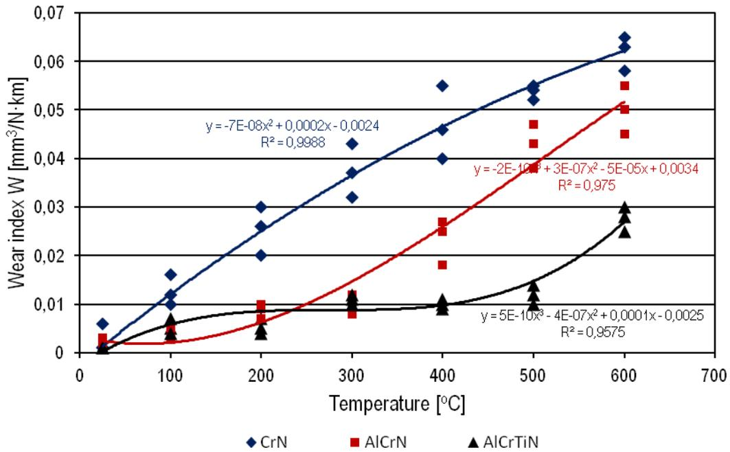
Fig.3. The results of ball-on-disc tribology tests obtained for three different investigated layer composites: PN+CrN, PN+CrAlN and PN+TiCrAlN.
