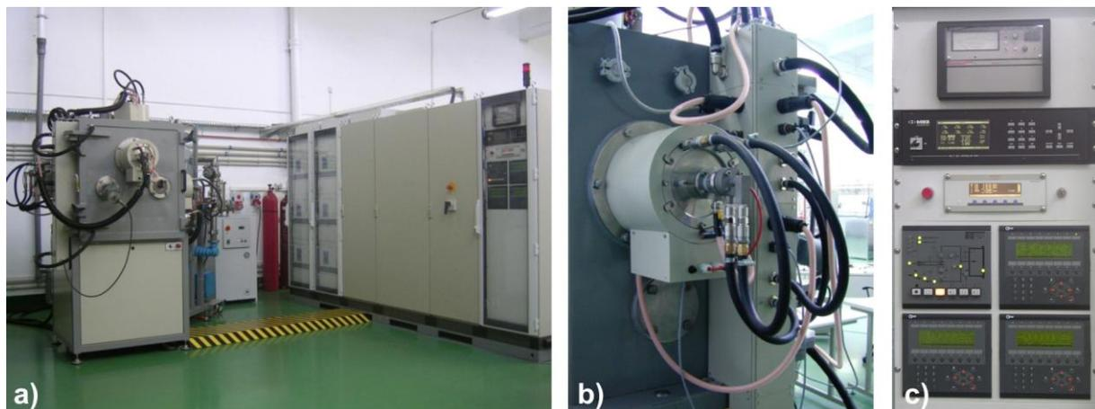
Fig.1. Device for the realisation of hybrid surface treatment processes a) entire technological system, b) arc plasma source, c) computer control system.
