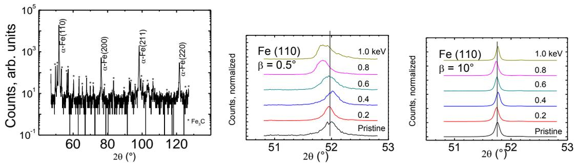
Figure 1. Left:  $\theta$ - $2\theta$  diffractogram of a typical sample. Middle:  $\alpha$ -Fe (110) x-ray diffraction peak for different Xe beam energies, taken at incident beam angle  $\beta=0.5^\circ$ . Right: incident beam angle  $\beta=10^\circ$ .
