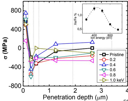
Figure 2. In depth stress distribution in the steel samples. The dotted vertical lines indicate the layers according to the model of constant average stress discrete layers used to deconvolute the stress profile. Here, each point represents the average stress in the respective layer. Inset: Xe/Fe (%) ratio for each bombarded sample as a function of ion energy.
