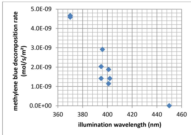
Figure 4: Methylene blue decomposition rate depending on illumination wavelength for comparable intensities (10 W/m<sup>2</sup> at 370 nm, about 10 W/m<sup>2</sup> at 400 nm, about 60 W/m<sup>2</sup> at 450 nm)
