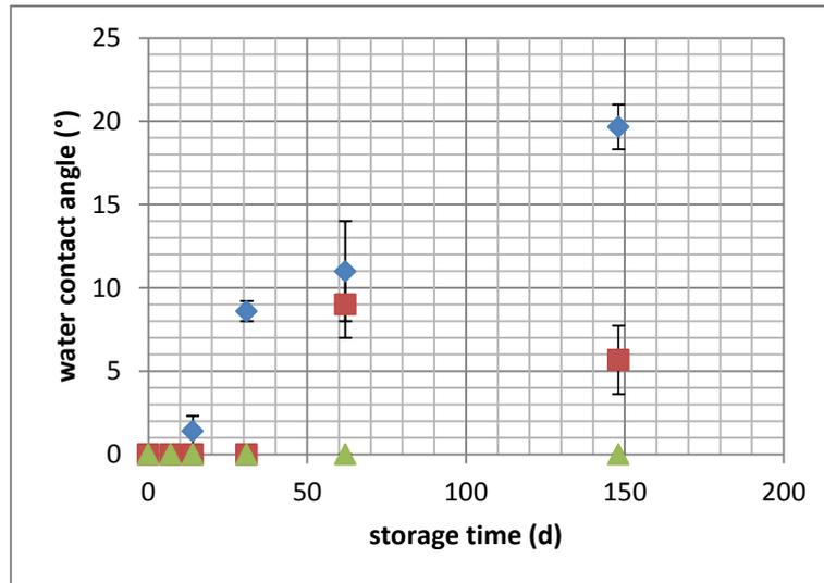
Figure 3: Water contact angle on TiO<sub>2</sub> coatings dependent on storage time in nitrogen gas (blue diamonds), distilled water (red squares) or physiologic saline (green triangles). Each point represents the mean value and standard deviation of three replicate samples.
