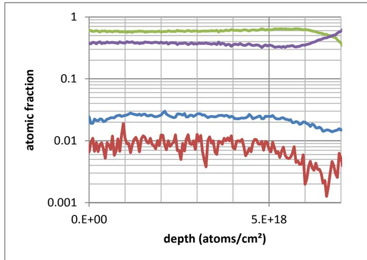
Figure 1: Atomic fraction of oxygen (green), titanium (violet), hydrogen (blue) and carbon (red) depending on depth in the coating obtained by ERDA. At a depth of  $7 \cdot 10^{18}$  atoms/cm<sup>2</sup> the titanium substrate is reached.
