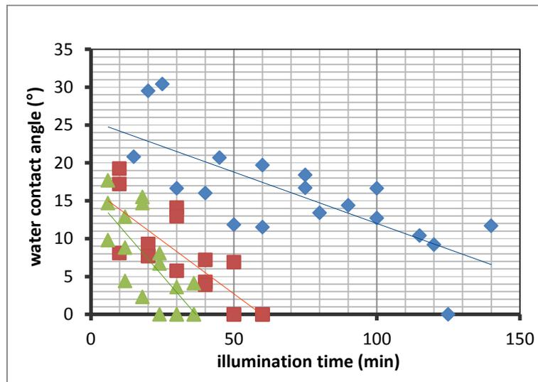
Figure 2: Water contact angle on TiO<sub>2</sub> coatings dependent on illumination time at wavelength 370 nm and intensity 5 W/m<sup>2</sup> (diamonds), 16 W/m<sup>2</sup> (squares) or 22 W/m<sup>2</sup> (triangles). For each intensity three independent experiments are combined in the graph. Lines are a guide to the eye.
