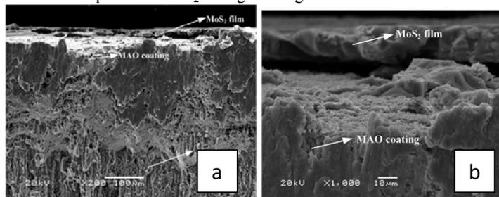
Fig.5 The sectional section micro-morphology of MAO coating with bonded MoS<sub>2</sub> films
