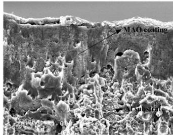
Fig.4 The sectional micro-morphology of MAO coating
