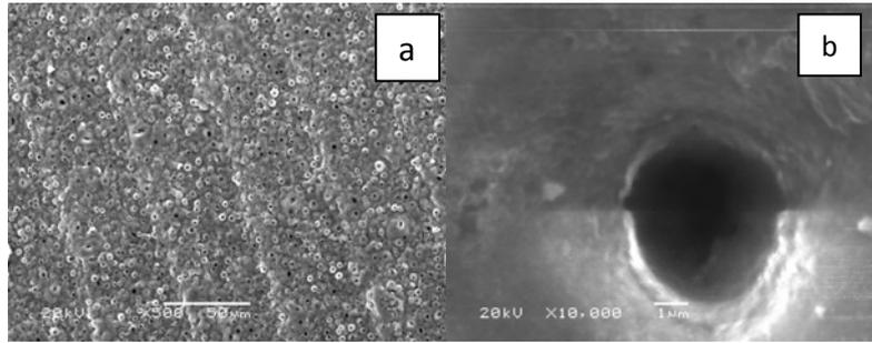
Fig.3 The microstructure of MAO coating with micro-pores
