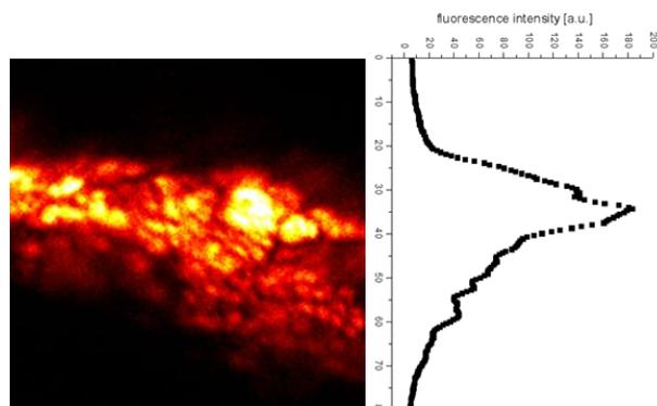
Fig. 6: Left – cross section image of labeled amino groups on a micro-tube membrane ( $80 \times 80 \mu\text{m}^2$ ), right- corresponding fluorescence intensity profile
