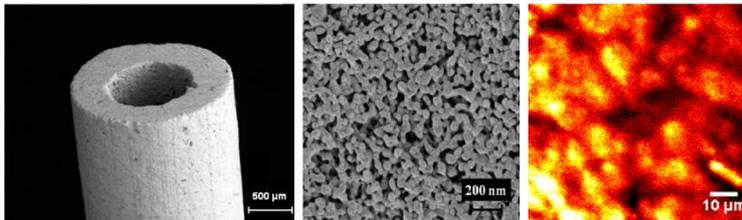
Fig. 4: Left and middle- SEM analysis of a ZrO<sub>2</sub> membrane in the overview (left) and in detail (middle)[8], right: Fluorescence intensity image of labeled amines on the membrane in µm resolution
