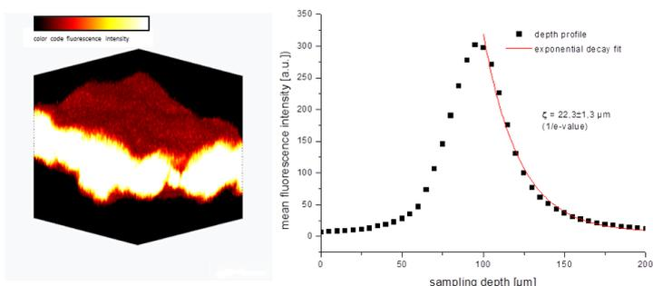
Fig. 5: Left – Rendered 3D image of labeled amino groups on a micro-tube membrane ( $80 \times 80 \times 205 \mu\text{m}^3$ ), right- corresponding fluorescence intensity depth profile
