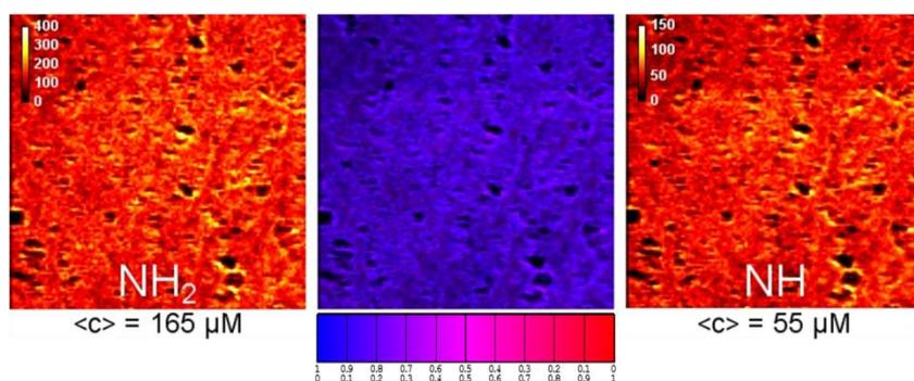
Fig. 1: Concentration distribution of primary and secondary amines on the top side of a plasma functionalized PP membrane after transferring intensities into concentrations via calibration curves [1]
