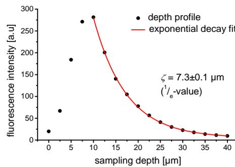
Fig. 3: Rendered 3D image of labeled amino groups after plasma treatment (left) and corresponding fluorescence intensity depth profile (right) with closed cavities setup [1]
