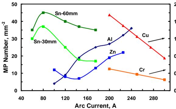
**Fig. 7.** Dependence of MP density on arc current for Sn (measured here), Zn and Al (left axis) and for Cu, Cr (right axis) [6,9], recessed cathodes. The substrate was exposed after 60 s for 15 s,  $L=110$  mm.
