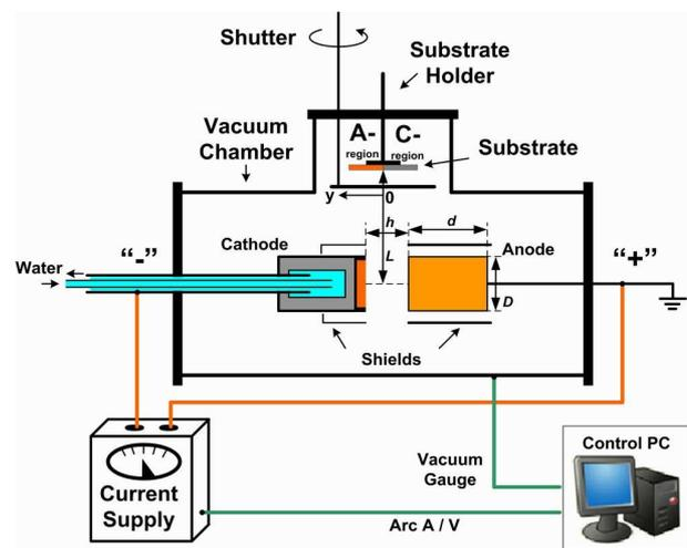
Fig. 1. Schematic diagram of the chamber, cathode-anode assembly and the substrate position with A and C regions.
