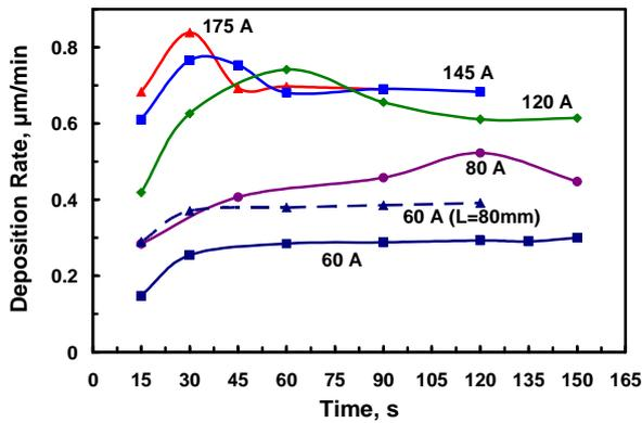
Fig. 4. Time-dependent rate of Sn film deposition,  $D=30$  mm cathode recessed 3 mm behind box shield,  $d=9$  mm graphite anode,  $h=10$  mm,  $L=110$  mm. (The case for  $L=80$  mm is also shown for  $I=60$  A).
