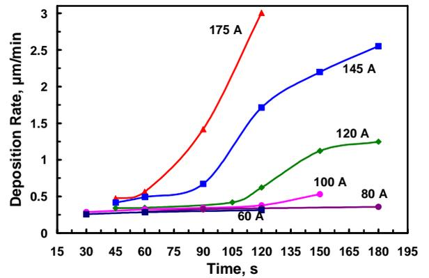
Fig. 2. Time-dependent rate of Sn film deposition,  $D=60$  mm cathode without shield,  $d=10$  mm W anode,  $h=10$  mm,  $L=125$  mm.
