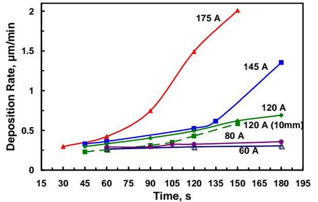
Fig. 3. Time-dependent rate of Sn film deposition,  $D=60$  mm cathode recessed 7 mm behind shield,  $d=10$  mm W anode,  $h=15$  mm,  $L=125$  mm. (The cathode recessed 10 mm behind the shield is also shown for  $I=120$  A).
