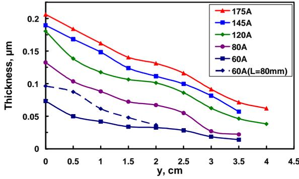
**Fig. 6.** Sn film thickness distribution in the A-region of the substrate in the  $y$ -direction from the A-C boundary with arc current  $I$  as a parameter.  $D=30$  mm cathode recessed 3 mm behind box shield,  $d=9$  mm graphite anode,  $h=10$  mm,  $L=110$  mm. (The case for  $L=80$  mm is also shown for  $I=60$  A).
