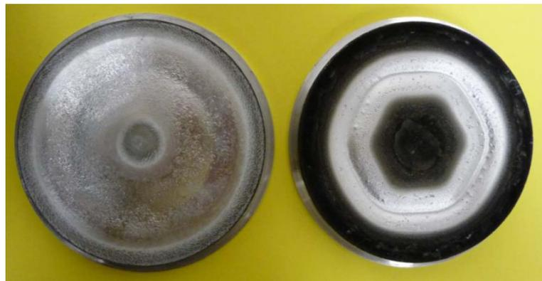
Fig. 1 View of the Al targets exploited in the GIMS (left photo) and under the condition of continuous working gas flow (right photo), respectively in the nitrogen only and Ar+N<sub>2</sub> atmosphere.
