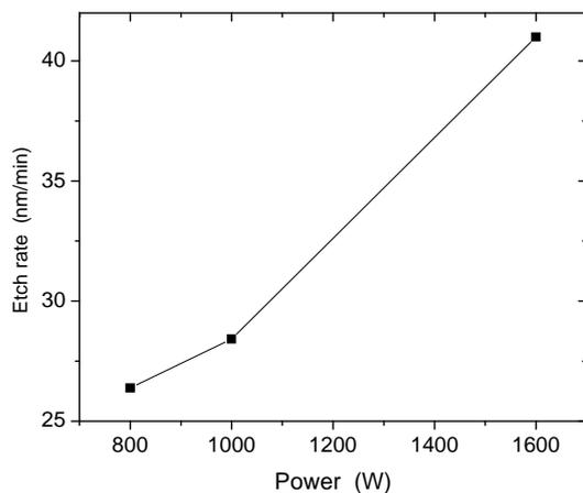
**Fig. 3** Dependence of etching rate of thin PMMA film on power forwarded to plasma. Etching conditions:  $p = 1$  Pa of H<sub>2</sub> with  $Q = 50$  sccm.
