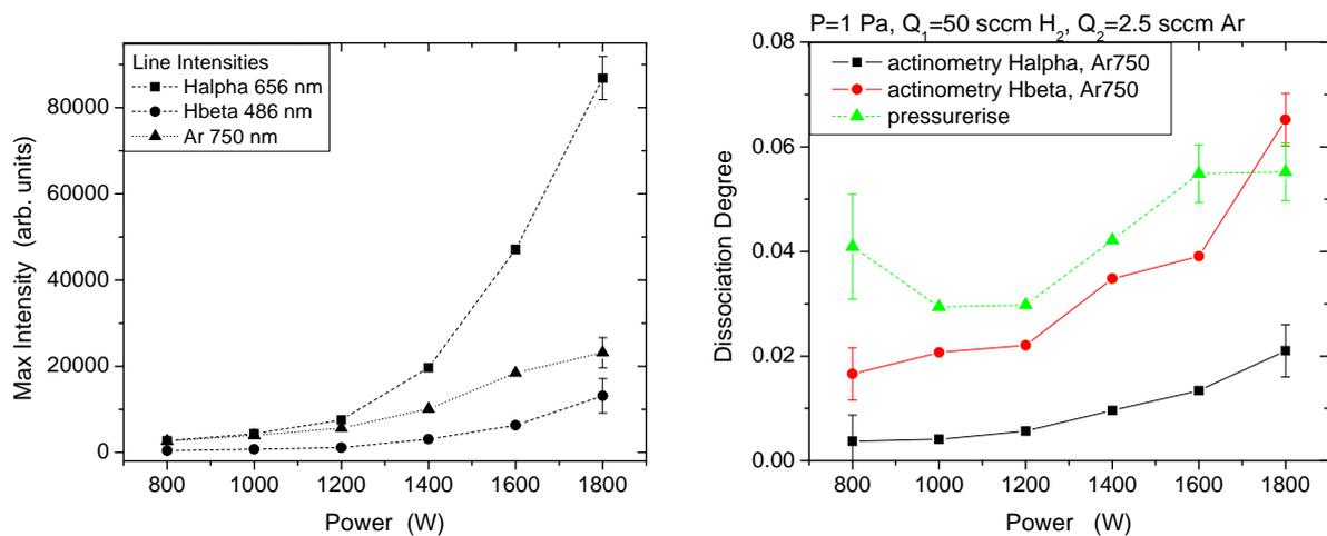
**Fig. 2** a) The dependence of peak line-intensity on power forwarded to plasma. Recordings done at  $p = 1$  Pa and  $Q = 50$  sccm. b) Change of the dissociation degree of  $H_2$  with power. H densities and dissociation degree were determined with actinometry measurements (shown with full lines calculated for  $T_e = 3$  eV), and pressure rise measurements (dashed line).
