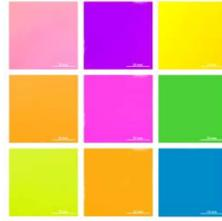
**Fig. 1:** Colour appearance of a Fabry-Perot stack ( $\text{SiO}_2\text{-Cr-SiO}_2$  on Al) with tilt effect; dependence on AOI and design features: normal incidence (upper line), AOI =  $45^\circ$  (centre line) and AOI =  $60^\circ$  (lower line); design A (left column), design B (centre column), design C (right column)
