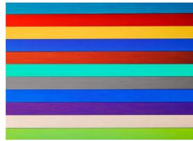
**Fig. 2:** Colour appearance of Fabry-Perot stacks without any tilt effect (Aradierung®)
