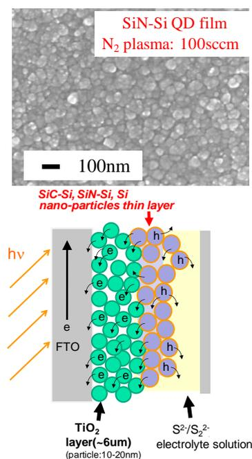
Figure 4. (a) SEM image of SiN nanoparticle films. (b) Cell structure of quantum-dot sensitized solar cells.
