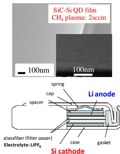
Figure 5. (a) SEM image of SiC nanoparticle films. (b) Cell structure of Li ion batteries.
