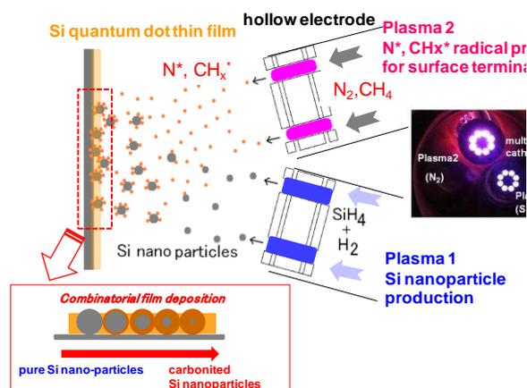
Figure 2. Schematic of experimental apparatus of double multi-hollow discharge plasma CVD.
