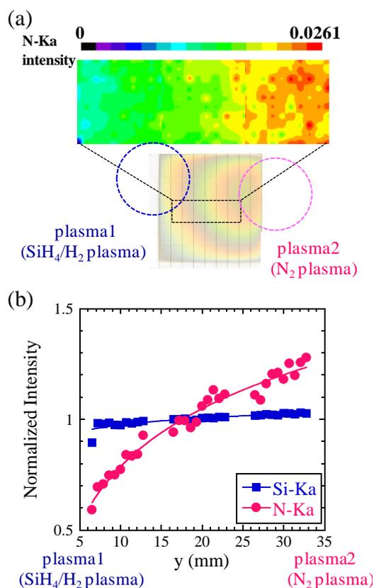
Figure 3. (a) Two-dimensional distribution of N-K $\alpha$  fluorescence intensity obtained from X-ray fluorescence (XRF) measurement. (b) Substrate position dependence of N-K $\alpha$  and Si-K $\alpha$  fluorescence intensities from XRF.
