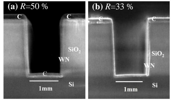
Fig. 4. Cross-section SEM images of (a) anisotropic deposition profile for  $R = 50\%$  and (b) top surface deposition profile for  $R = 33.3\%$ .
