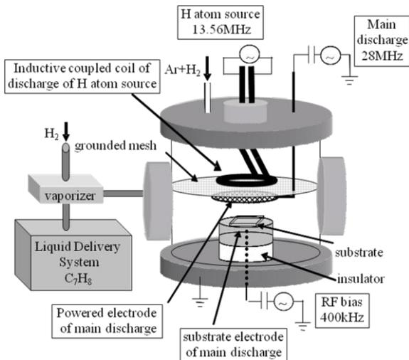
Fig. 1. H-assisted plasma CVD method.
