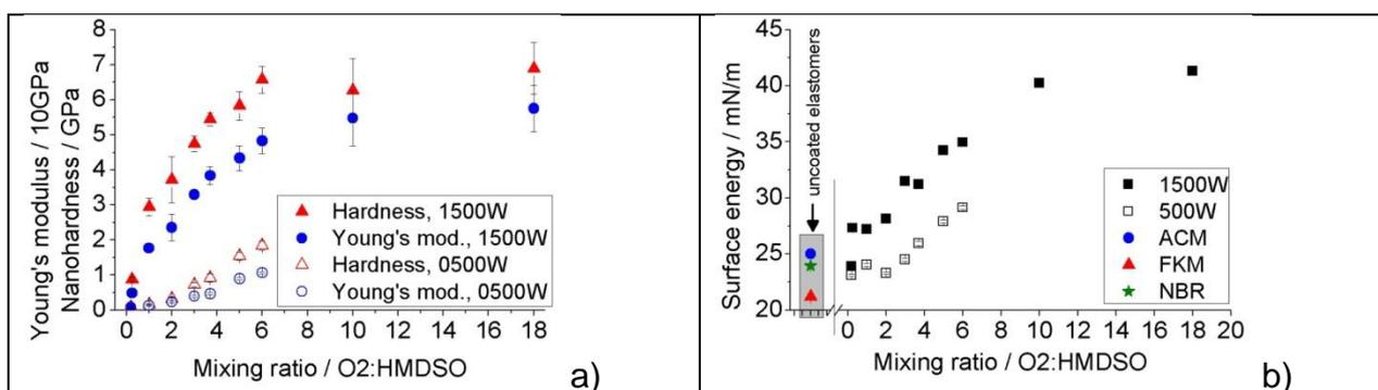
**Figure 2:** a) Young's modulus and nanohardness of the plasmapolymeric coatings varying the mixing ratio of the process gases. b) Surface energy of elastomeric substrates and plasmapolymeric coatings. The surface energy of the plasmapolymeric coating could be tailored varying the mixing ratio of the process gases.
