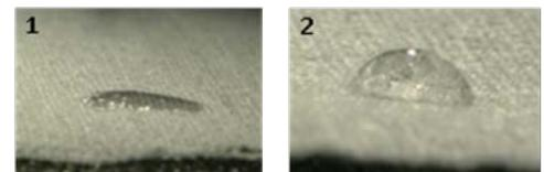
Table 1: LOI and Schermer pressures ( $P_{Sch}$ ) before ( $LOI_1/P_{Sch1}$ ) and after ( $LOI_2/P_{Sch2}$ ) the  $CF_4$  plasma treatment on untreated- and FR-cotton fabrics and photographs of droplets of water on FR-cotton before (1) and after (2)  $CF_4$  plasma treatment.
