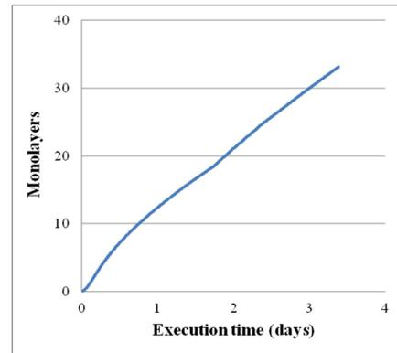
Fig. 4. Evolution of system size with execution time at T=180°C (dilution ratio=3% SiH<sub>4</sub>).
