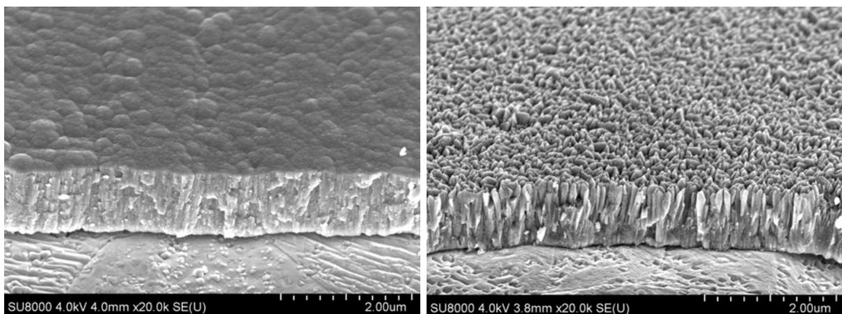
**Figure 2** Titanium dioxide coatings on steel strip, SEM images of cross fracture, amorphous (left) and anatase phase (right)
